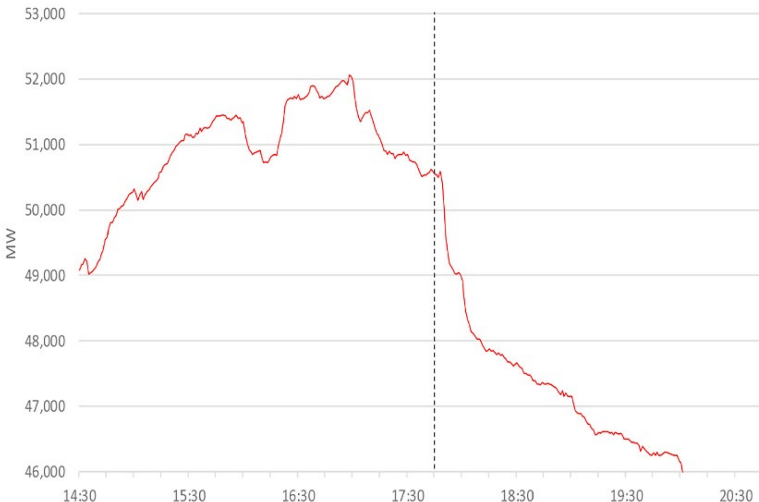
Last-minute customer conservation measures sharply reduced California’s electricity demand during strained grid operations on Sept. 6, 2022, averting the need for rolling blackouts. | CAISO
